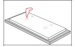
When installing with a countertop, offer the countertop to the wall mounted units and mark the position of the waste and tap holes. Place the countertop on top of a surface such as MDF and make the required holes. All holes made into wood should be sealed with a PVA or
